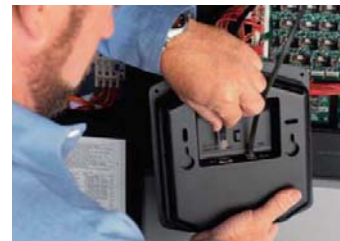
Removable display makes servicing easier
